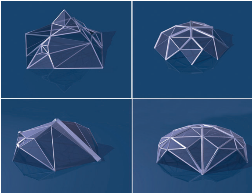
◀ Figure 7. Dome shapes generated with eifForm software
