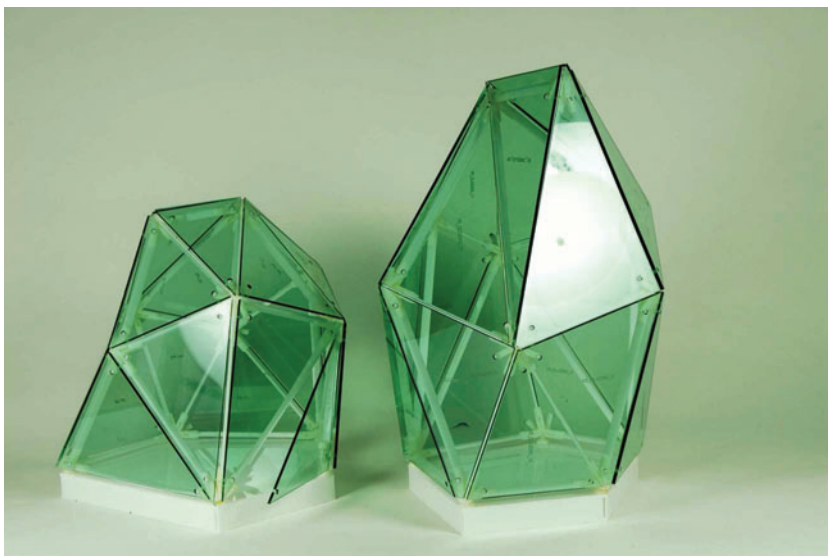
◀ Figure 14. Parametric variation of the same geometry both manufactured from laser cut acrylic and FDM modeled plastic assembly clips.
