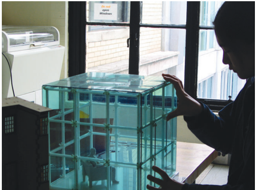
► Figure 3. Physical assembly of elements manufactured with a rapid prototyping device and laser cutter
