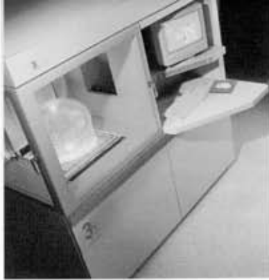
3.19. The SLA 250 stereolithography system by 3D Systems.
