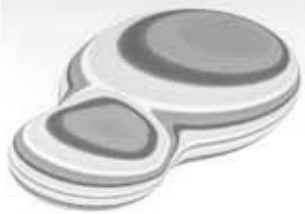
3.58. Gaussian analysis of a doubly-curved surface.
