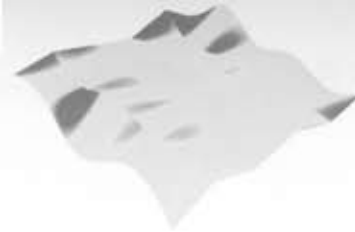
3.59. Gaussian analysis of a developable surface.
