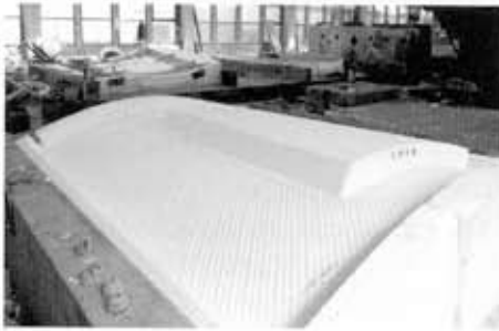
3.17a–f. The reinforced concrete panels for Gehry's Zollhof Towers (2000) in Düsseldorf, Germany, were precast in CNC-milled Styrofoam molds.
