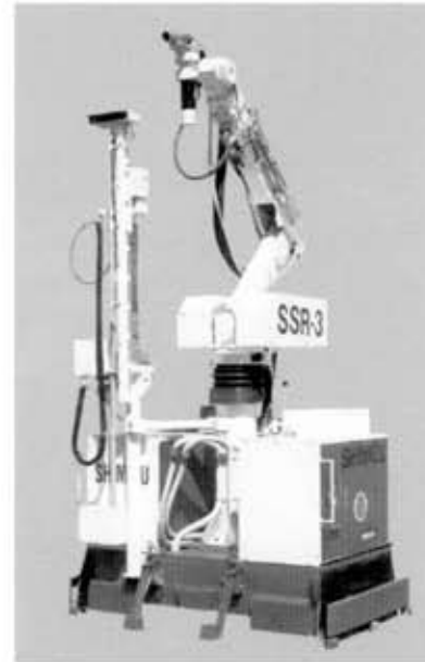
3.27. Shimizu's Insulation Spray Robot .
