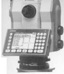
3.25. Trimble's 5600 Series Total Station advanced surveying system.
